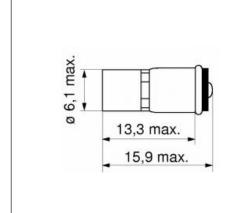
Part Number: 1510135UR3 Serial Number: 15101 Based LED type: StarLED Size (inch): T-1 3/4 Size (mm): T6
