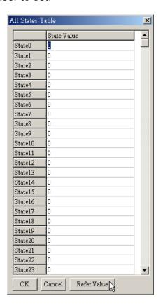
Step 7. "Refer Value" can be used to calculate state range.
