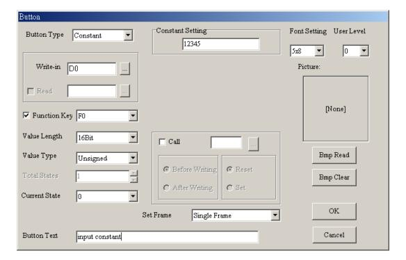
Increase/Decrease: Pressing this button and GP will read register data from ELC and add or submit according to the settings. It will write the result to ELC corresponding register. If you set 10 for inc/dec and 1000 for up/down bound, it means it will increase/decrease 10 for each time you press the button. And the maximum you can increase/decrease is 1000.
