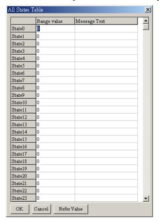
Step 6. "Refer Value" can be used to calculate state range.
