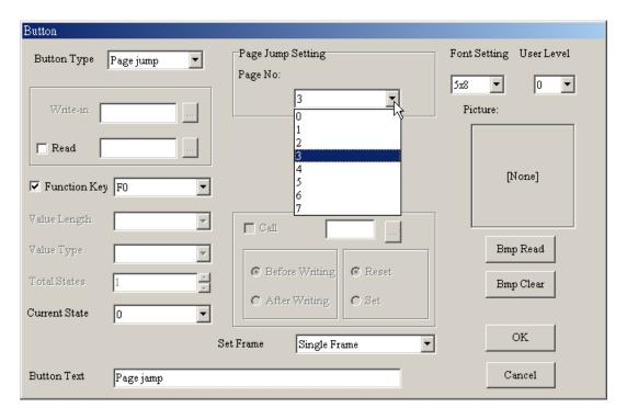
Password: There are functions of password setting and inform command in the dialog box. You could use password setting to protect this button. And you could check "call" to set to call the reference device to reset to set before writing or after writing. User can use "User level" to set the user priority.
