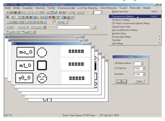
After entering the correct settings, the PC is capable of communicating to the GP.
