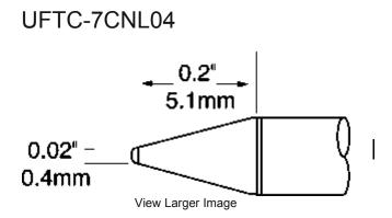
UltraFine Tip Cartridge, Conical, Long, 0.4mm x 9mm, 700 series, for use with the Metcal UltraFine hand-piece (MX-H2-UF)
