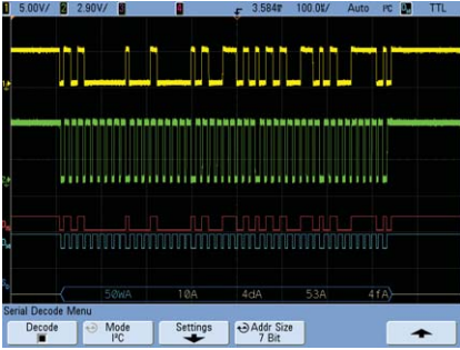
View on-screen serial decode of an I 2 C packet.
