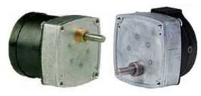
The PA and PB geared motors are the work horses of the Hurst product line. All gears are hobbed to AGMA 7 standards. Pinions are extruded from a special steel with a modified long addendum tooth form to provide higher strength. Both pinions and gear teeth are case hardened and rotate upon hardened and ground steel studs. Synthetic lubrication is used throughout.
