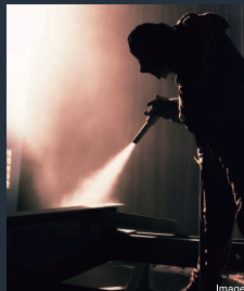
IP69K (80°C Jet-stream Steam Examination) (Standard Number / DIN 40 050-4)
