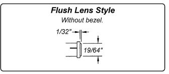
Flush Lens Variety of Lens Colors 1/8" Tab Terminals or 3/16" Tab Terminals PressFit Mounting
