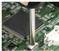
Cartridge handpiece with rework tips for SMD rework
