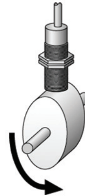
Eccentricity or Absolute Angle Detection
