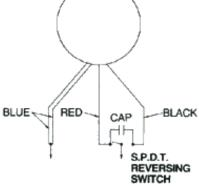
Current applied to the blue and red leads produces CW rotation. Switching the current to the blue and black leads produces CCW rotation. For dual speed versions switching the current produces a change in speed but not in direction of rotation. Direction of rotation must be specified separately.
