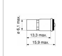
Part Number: 1510145UR3 Serial Number: 15101 Based LED type: StarLED Size (inch): T-1 3/4 Size (mm): T6
