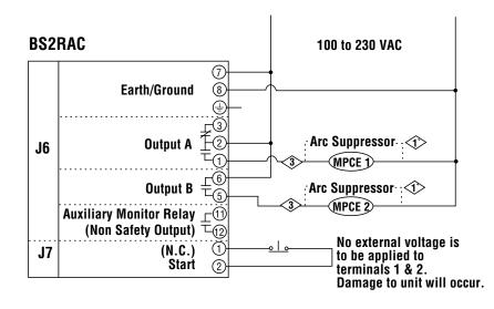
Normally Open/Normally Closed Connection Diagram
