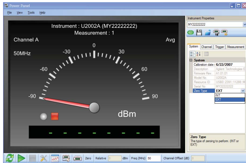
Figure 1: Setting External Zeroing (EXT) in the N1918A Power Panel
