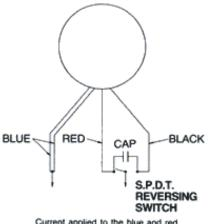
Current applied to the blue and red leads produces CW rotation. Switching the current to the blue and black leads produces CCW rotation.
