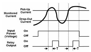
than the adjustable time delay of 0.1-10 seconds. This delay prevents nuisance tripping caused by inrush currents. It will de-energize when the monitored AC current is below the drop-out setting.
