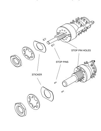
The adjustable stop Series 71 rotary switches allow you to change the number of positions per pole. Simply remove and relocate stop pins in the holes in the front of the switch. The pins are held in place by a self adhesive sticker which fits over the front plate.
