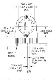
Note: Common location for a single pole per deck switch. For common location on two pole switches see circuit diagrams.
