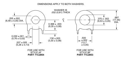
For printed circuit styles. Mounting bushing provides additional support for the front end of the switch. Order separately by appropriate part number. Rotary switch discount applies.
