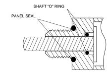
The shaft is sealed by an O-ring inside the bushing. The panel is sealed by an O-ring at the base of the bushing.
