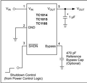
The TC1014/TC1015/TC1185 are high accuracy (typically  $\pm 0.5\%$ ) CMOS upgrades for older (bipolar) Low Dropout Regulators (LDOs) such as the LP2980. Designed specifically for battery-operated systems, the devices' CMOS construction eliminates wasted ground current, significantly extending battery life. Total supply current is typically 50  $\mu$ A at full load (20 to 60 times lower than in bipolar regulators).
