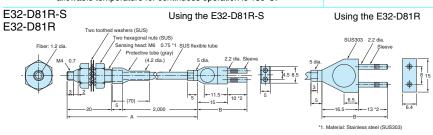
Note 1. The maximum allowable temperatures for sections A and B are 200°C and 110°C, respectively. The section inserted into the Amplifier Unit (indicated by \*2), however, must stay within the Amplifier Unit's operating temperature range.
