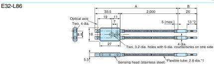
Note: The maximum allowable temperatures for sections A and B are 200°C and 110°C, respectively. The section inserted into the Amplifier Unit (indicated by \*2), however, must stay within the Amplifier Unit's operating temperature range.
