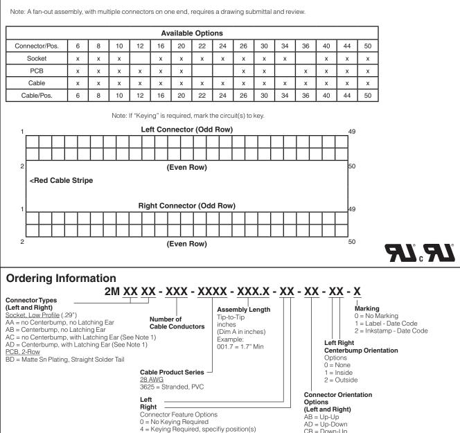
Notes: 1. Latching ear option is required for mating with the 3M<sup>™</sup> Latch/Eject Header 2 mm, 1552 Series 2. (RIA E1 & C1 apply for all cables and connectors listed)
