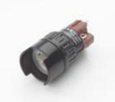
Illuminated pushbutton, snap-action, raised, round, black plastic, 16mm mounting, solder terminals, gold over silver contacts
