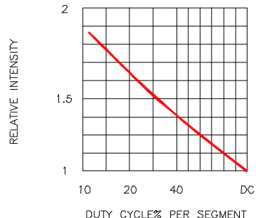
Fig.4 LUMINOUS INTENSITY VS. DUTY CYCLE
