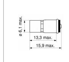
Part Number: 1510125UG3 Serial Number: 15101 Based LED type: StarLED Size (inch): T-1 3/4 Size (mm): T6
