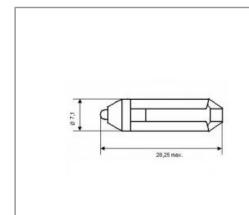
Part Number: 1508635W3D Serial Number: 15086 Based LED type: StarLED Size (inch): T-2 Size (mm): T7
