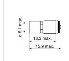
Part Number: 1510135W3D Serial Number: 15101 Based LED type: StarLED Size (inch): T-1 3/4 Size (mm): T6
