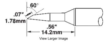
Bevel style, 1.78mm, 60 degree, soldering cartridge, 700 series, for use with MX-RM3E Rework Hand-piece or MX-H1-AV Metcal Advanced Hand-piece
