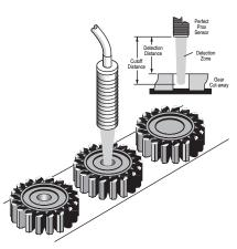
If the hole is If the hole is present in the gear, the sensor will shine through the hole and ignore the belt — no detection event will occur.
