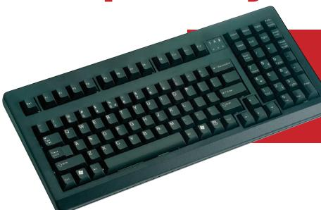
Durable Compact Keyboards with Mechanical Keyswitch Technology for Industrial and Commercial Aplications
