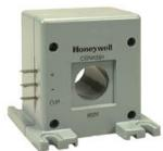
CSN Series closed loop current sensor, measures ac, dc or impulse current, 300 A nominal, ± 600 amp range, busbar, 2000 turn
