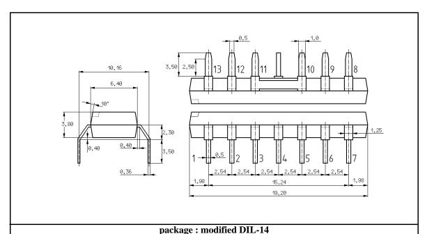
1, 2, 7: not connected 3:  $+V_O$  4:  $-V_B$  5:  $-V_O$  6:  $+V_B$  8, 9, 10: current output 11, 12, 13: current input  $V_O$  - output voltage  $V_B$  - supply voltage
