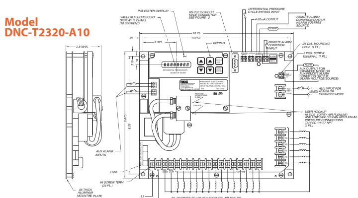
SOL. COM. TERMINALS ARE INTERNALLY CONNECTEDTO L2 TERMINAL
