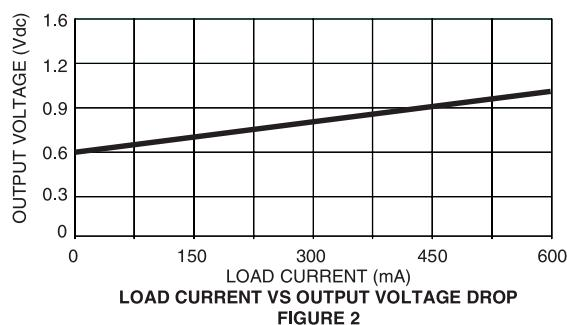
LOAD CURRENT VS OUTPUT VOLTAGE DROP
