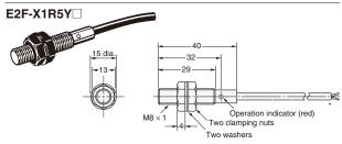
\* 3.5-dia. vinyl-insulated round cable with 2 conductors (Conductor cross section: 0.14 mm², Insulator diameter: 1 mm), Standard length: 2 m
