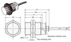
\* 6-dia. vinyl-insulated round cable with 2 conductors (Conductor cross section: 0.5 mm², Insulator diameter: 1.9 mm), Standard length: 2 m
