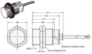
\* 6-dia. vinyl-insulated round cable with 3 conductors (Conductor cross section: 0.5 mm², Insulator diameter: 1.9 mm), Standard length: 2 m
