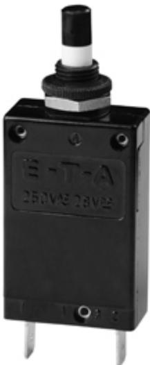
Single pole thermal circuit breaker with press-to-reset, tease-free, trip-free, snap action mechanism. Type 2-5700 can be supplied as a push-push switch/circuit breaker (R-type TO CBE to EN 60934 in press-to-reset configuration; S-type with push-push operation), threadneck panel mounting. Options include an additional unprotected circuit tap (-A3). Approved to CBE standard EN 60934 (IEC 60934).
