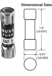
Catalog Symbol: BAF (5AG) Fast-Acting 2/10 TO 30 UL Recognized, STD. 248-14 0-15/250Vac (GUIDE # JDYX, FILE # E19180) CSA CERTIFIED 0-15/250Vac (CLASS 1422-01, FILE # 53787)
