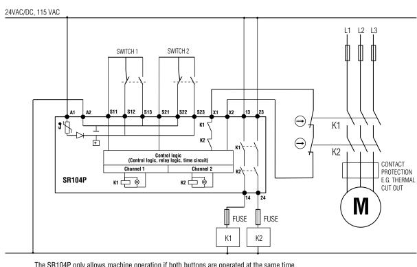
The SR104P only allows machine operation if both buttons are operated at the same time. Operating one button or both buttons and then releasing one will not start the machine.
