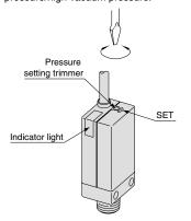
• Set the possible min. pressure for adsorption confirmation. If setting the pressure lower than that, switch becomes ON in case that adsorption is not completely done. If setting the pressure higher than that, switch does not become ON even though it may absorb workpieces.
