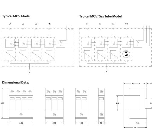
Mounting: Symetrical rail EN50022/DIN 46277-3 I/O Connections: By screw terminal 4-25mm<sup>2</sup> by connection bus
