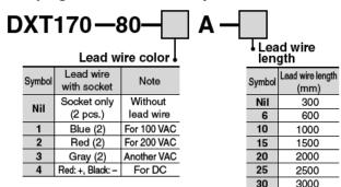
Note) When ordering a valve in which the length of the wire is more than 600 mm, be sure to indicate the model number of valve without connector and connector assembly.
