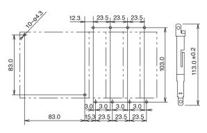
Mounting hole layout from left, FC4A-HPH1, FC4A-D20K3, FC4A-N16B3, FC4A-N32B3, and FC4A-M24BR2 modules
