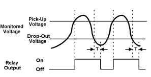
setting. The relay de-energizes when the monitored voltage is below the drop-out setting for a period longer than the drop-out time delay (T), which is adjustable from 0.5-10 seconds for VA Series products. A time delay on drop-out fixed at 500ms is available (see Page 25).
