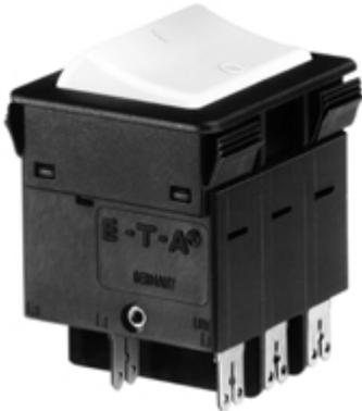
Single, two and three pole rocker switch/thermal trip free circuit breakers (S-type TO CBE to EN 60934) of compact design for snap-in panel mounting. Available either with protection on one/both/all poles or, in the case of the double pole version, protection on one pole only. Illumination is optional and there is a choice of rocker colours. Approved to CBE standard EN 60934 (IEC 60934).
