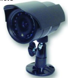
This camera is a part of Speco Technologies' Value Line. It is a color day/night camera with built-in 4mm lens, 10 IR LEDs, CDS sensor in a plastic waterproof case. Sunshield, mounting bracket and 12 Volt DC regulated power supply are included.
