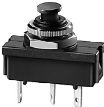
Single pole press-to-reset thermal circuit breaker with extremely fast overload switching performance (R-type TO CBE to EN 60934). Single hole threadneck mounting. Type 1410-G1 features changeover contacts suitable for providing status output signals. Largely temperature-insensitive.
