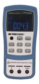
The Model 830B Capacitance Meter's large  $4_{1/2}$  digit LCD dual display can simultaneously display values and deviations from selected tolerances. The unit can also sort on preset tolerances of 1, 5, and 10%. The built-in chip and microprocessor allows the user to program unique values to sort specific circuit applications. Outstanding features of the Model 830B include:
