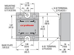
Screw Torque Requirements: 6-32 Screws - 10 in. lbs., 8-32 - 20in. lbs. (Screws dry without grease.)
