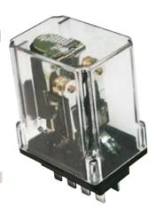
The 21 series coil is rectified which provides chatter free operation in brownout conditions down to 85VAC and will not overheat up to 130VAC. Rectified coils also provide less power consumption and less heating.
