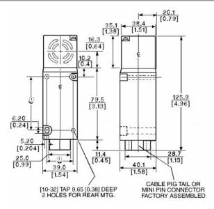
$^{\scriptsize\textcircled{1}}$  Can accommodate both U.S., 29.4 [1.16] x 59.5 [2.34] and DIN, 30 [1.18] x 60 [2.36], mounting dimensions.
