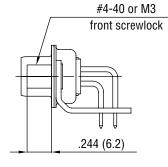
Fixed front female screwlock VF / VFM
