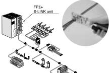
2. Up to four units can be connected. Each unit can control up to 128 I/O points.
