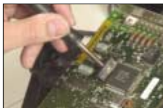
A SMT blade tip is ideal for soldering the leads of a QFP.
